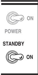
Wait at least 30 seconds and then flip the **STANDBY** switch to the ON position. This prevents tube problems and increases their toneful life substantially.
